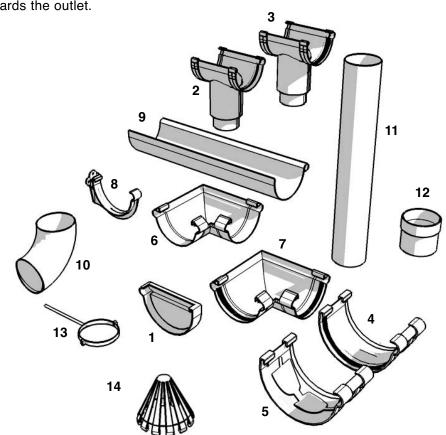
Determine the position of the outlet. That is automatically the lowest point. After that, you can also determine the highest point. Install a bracket at the lowest and one at the highest point. A string secured between both brackets will assist in installing the remaining brackets.
