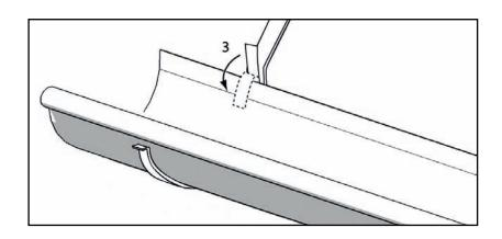
If you use glue-fittings, the gutter can be glued into the fittings. Make sure the surface is clean before applying the glue. The seam in which the gutter is stuck, must be filled with glue. Afterwards, apply some additional glue along the inside seam.
