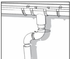
With elbows you can guide the downpipe from the gutter outlet to the wall. Connect the downpipe and elbow by using glue.
