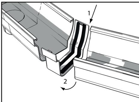
If you use rubber fittings, the gutter can be stuck into the fittings. First you 'click' the backside of the gutter into the fitting (1), then the frontside (2). Markings on the inside indicate the gap that must be left to accommodate thermal movement.
